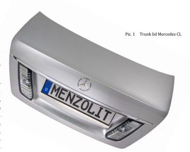
benefits and ease with the integration which Menzolit SMC 0430 provides, optimizes design and creates subsequent savings in assembly. The grade exhibits good moulding attributes which results in surface defect free body parts when moulded under constant moulding parameters and practices. After application of a conductive primer, electrostatic coating is possible both online as well as offline.
