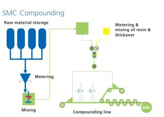
On the SMC continuos line the doctor box delivers paste onto a carrier film. The cutter adds a layer of chopped glass fibres on top of the paste. Then paste is metered on a second film, fed on top of the glassfibres to form a sandwich of paste/fibres/paste.
