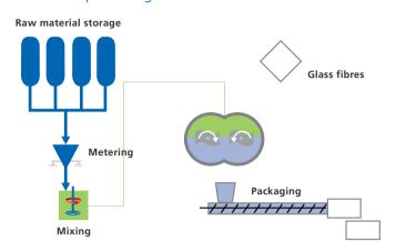
BMC is prepared in a mixer. After preparing a base paste it will be loaded into the mixing device. Then all other ingredients are added and homogenized. BMC is packed into bags until moulding. To avoid any material changes during storage and transport it is packaged in a styrene tight packaging.
